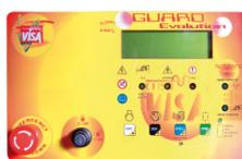
The **GUARD EVOLUTION** device, in MANUAL or AUTOMATIC version, is designed and manufactured by Visa S.p.A. for the command, control and protection of the generating set. Main characteristics are: clear communication via a large backlit display screen; generating set event analysis through sophisticated algorithms; complete engine and electrical parameters; possibility of integrating additional modules and programme extensions; customisation for dealers (optional).
